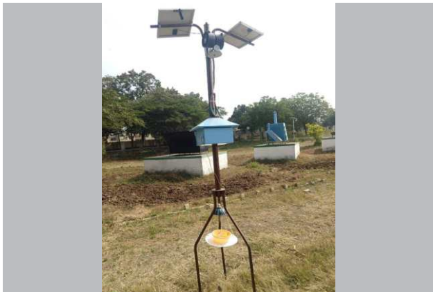
Solar operated animal/bird scarer cum light insect trap
