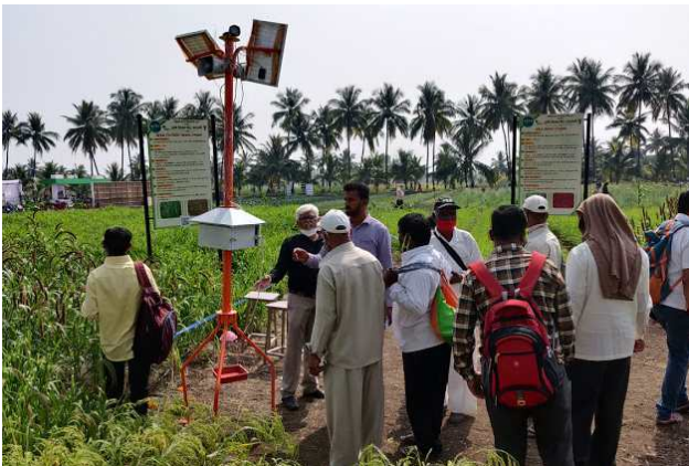
Solar operated animal/bird scarer cum light insect trap
