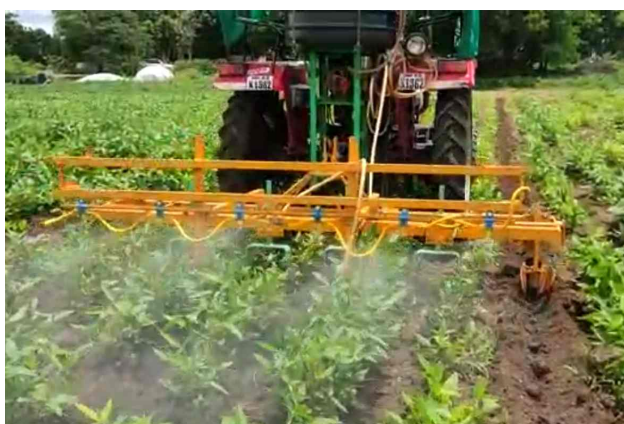
Tractor Drawn Inter- Cultivator Cum Sprayer For Soybean and Cotton with slim tyres
