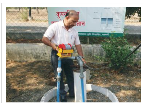
Measurement of ground water levels in bore well using water level indicator in May, 2015 at Dryland Research Station, VNMKV Parbhani
