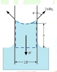
The upward force supporting the column of water is surface tension, while the weight of water column is the opposing force which tends to pull the water column down.
