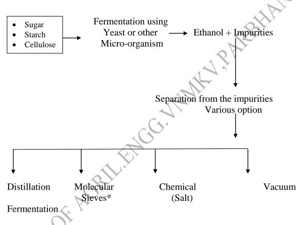
\*Today, almost all ethanol plants use molecular sieves for dehydration. The technology alone reduces energy use by 10 per cent per liter of ethanol produced.
